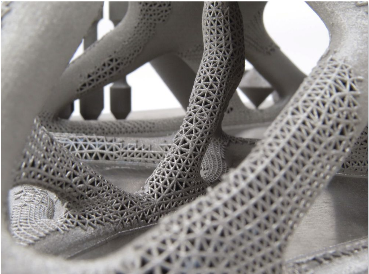
Altair's topology optimization software has a symbiosis with additive manufacturing, maximizing design freedom to create complex, freeform "bionic" structures. Image courtesy of Renishaw.
