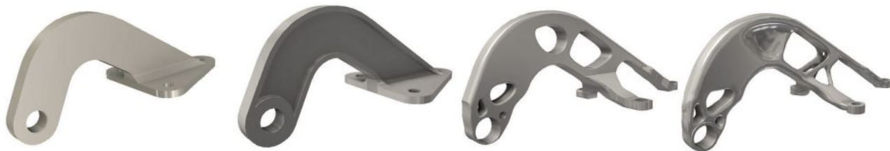
Four stages of lightweighting a bracket: simulation and analysis performed with the new Shape Generator feature in Autodesk Inventor. Users define part material, apply loads, identify fixed points and enter a value for the amount of mass to be removed. Image courtesy of Autodesk.
