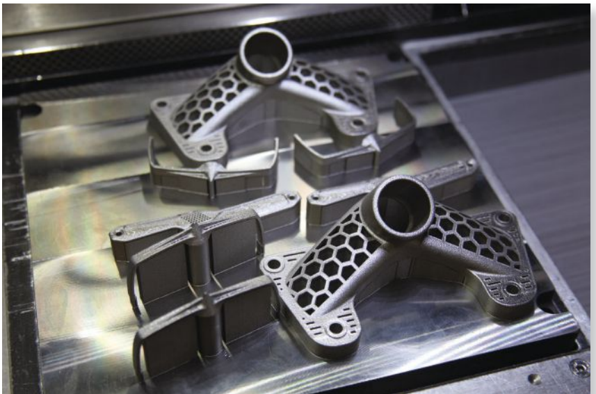
Stratasys Direct Manufacturing's Direct Metal Laser Sintering (DMLS) offerings are helping optimize structures for aerospace applications, including this lighter weight bracketed part. Image courtesy of Stratasys.
